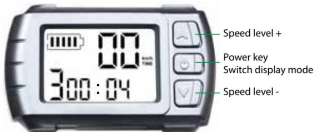
Display mode: ODO, VOL, TIME, DIS, RPM
