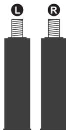
The enclosed Allen key is used to adjust the brake and manual accelerator pedal. To do this, turn it counterclockwise, set the desired position and turn it clockwise.
