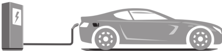
Fig. 3-2 Schematic diagram of CASE C connection
